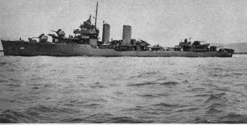
MACDONOUGH of the Farragut Class looks like the pre-war British DD's. Unequal square-topped stacks, straight deck lines are typical.
